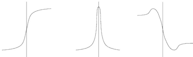
*Example: the intensity function around a step edge and its first and second derivatives.*
