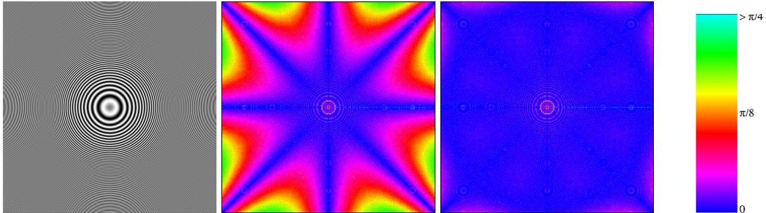
Figure 2: From left to right: test image with  $I = \sin(r^2)$  ; Sobel 3x3 angle errors; Scharr 3x3 angle errors; error colors.
