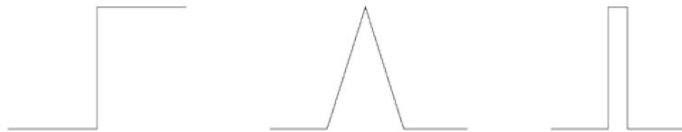
*Different types of edges: step, peak, roof.*
