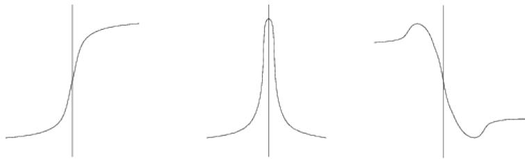
*Example: convolution of a step edge intensity function with a Gaussian and its first and second derivatives.*
